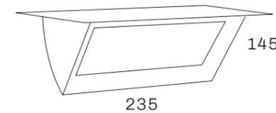
Recessed LED wallwasher with a very wide beam angle. Ideal for lighting wall presentations. Powder coating finish. Glass standard included. Equipped with Philips Fortimo LED module and Philips Xitanium LED driver.
