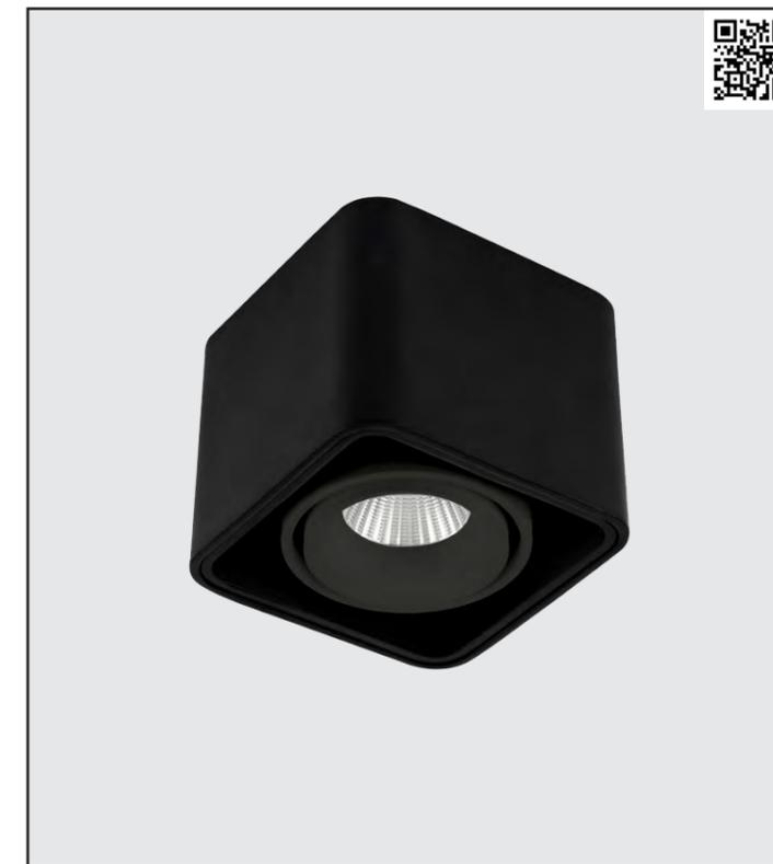
Surface mounted 30° tiltable cardanic spotlight with powder coating finish. Standard IP44, equipped with a Dim-to-Warm LED module and Triac dimmable driver.
