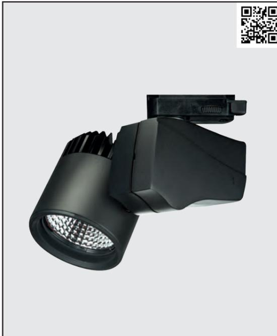
Compact 3-phase aluminium tracklight with passive cooling body and driverbox. Powder coating finish. Equipped with Philips Fortimo LED module and Philips Xitanium LED driver.
